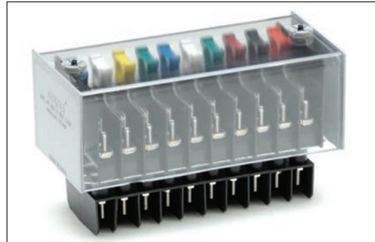
Nonslotted, back-connected clear cover – The nonslotted covers for back-connected switches fit flush with the panel because all wiring exits at the rear of the test switch
