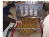
微波烘干黄粉虫 Microwave drying of TetraBiol molitor
