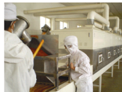
辣椒粉烘干杀菌 Chili powder drying and sterilization
