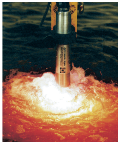
Underwater plasma cutting with FineFocus 800 / 1600
