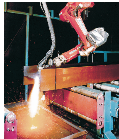
Plasma Cutting in combination with a robot with FineFocus 450 / 800
