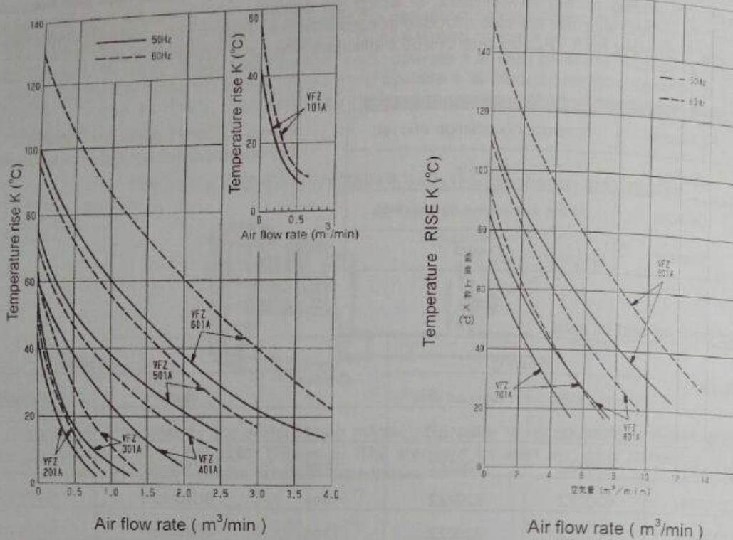
(Figure 6) Discharged air-temperature rise curve
